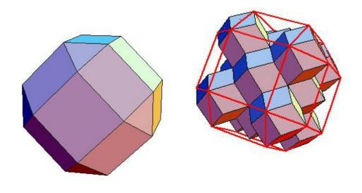
Observing triangular faces of the rhombic cuboctahedron we observe a deficit of 1/4 of the tetrahedron at each. Each rectangular face lacks two quarters of rhombic dodecahedron and square face lacks four eights of the rhombic dodecahedron. So to obtain the best approximate these parts of rhombic dodecahedron should be added.
