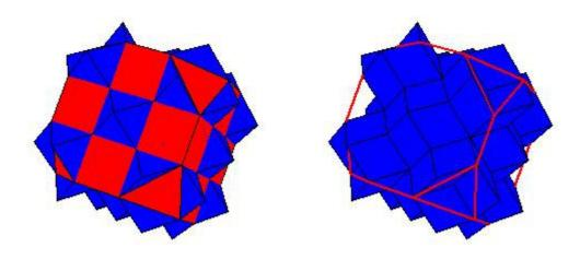
Observing triangular faces of the truncated cube we see a surplus of 1/4 of the tetrahedron at each face. At octagonal faces we observe a surplus of four eights and one half of the cube and a deficit of four halves of the cube. This gives a deficit of one half of the cube for each face. This means that we should add 3 small cubes (or 3/2 of rhombic dodecahedron) to obtain the best approximate of truncated cube.
